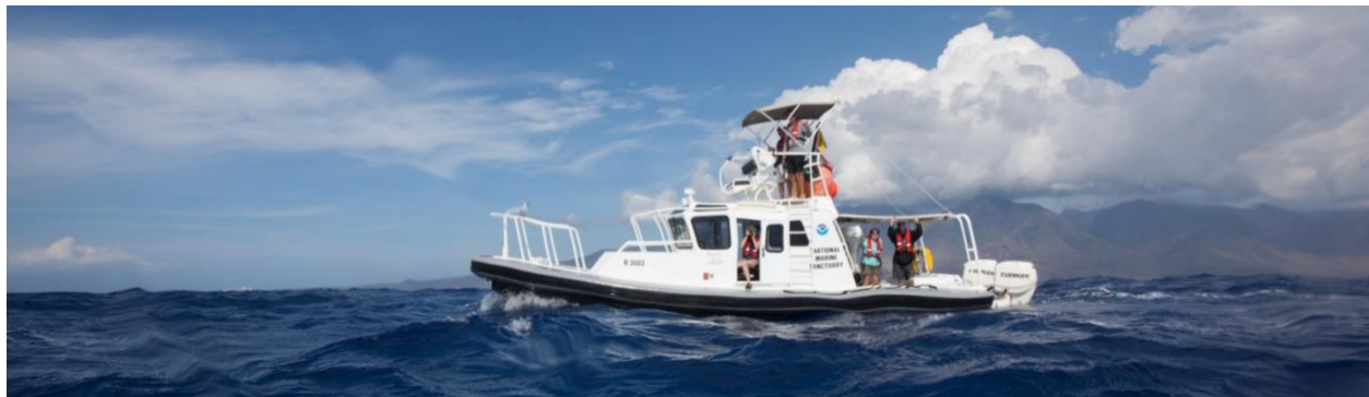
Hawaiian Islands Humpback Whale National Marine Sanctuary operates the R/V Koholā , a 38-foot rigid hull inflatable boat specifically designed for large whale research and entanglement response. Photo: Jason Moore/NOAA, under NOAA Permit #15240
